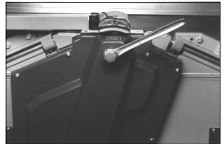
To assist in manually turning the cutterblock, remove the lid and place a 24 mm socket wrench on the cutterblock nut (wrench not supplied with the tool set).
